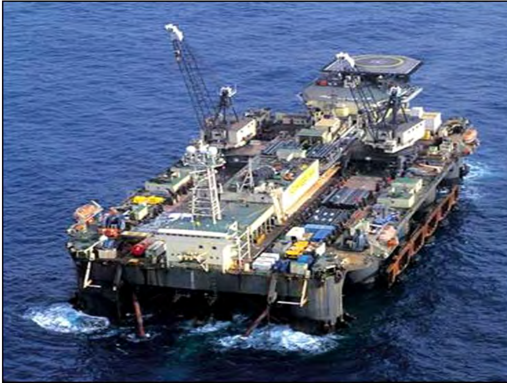
Figure 6-13 Castoro-Sei pipe-laying vessel.
