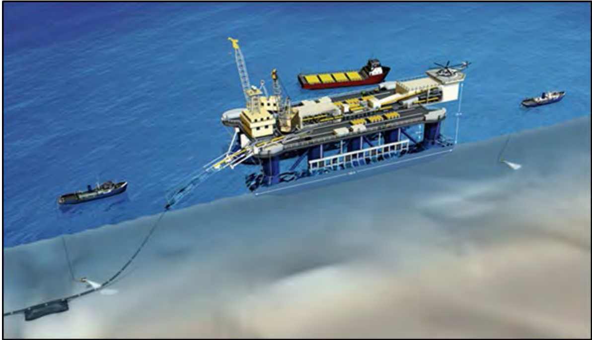
Figure 6-11 The S-lay pipe-laying vessel and survey support vessels.
