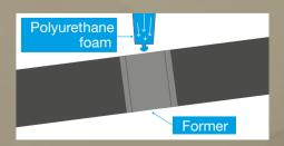
Once the weld is confirmed O acceptable, a corrosion resistant, heat-shrink sleeve is applied over the circumferential girth weld. Then, polyurethane foam is poured into a former surrounding providing further protection.
