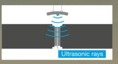
4 The double-joint is moved to a non-destructive testing station where every millimetre of the weld undergoes automatic ultrasonic testing (AUT) to detect any unacceptable flaws. If required, the defect will be removed and the weld rescanned to ensure it meets international standards.
