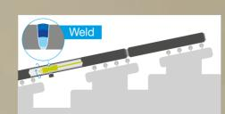
C The double-joint is now joined O to the end of the pipeline using a semi-automatic welding process. welding is performed in accordance approved welding procedures.
