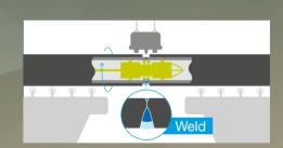
B Here, 12-metre pipe joints are aligned and welded together to create a double-joint segment measuring 24 metres. These sections will later be connected to the main
