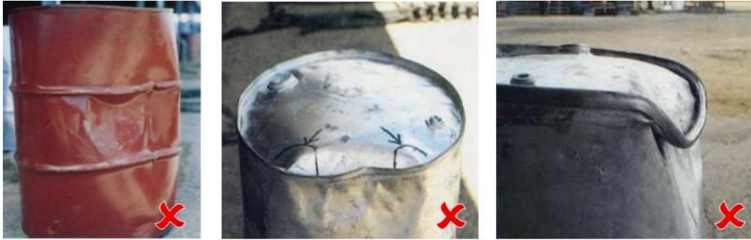
Sharp indents and damage to the edges or rolling hoops are potential leak points
