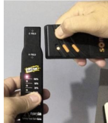
Then testing the RF EME meter which is calibrated to the general public limit
