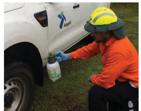
Plant and equipment need to be disinfected before entering bushland or leaving infested areas
