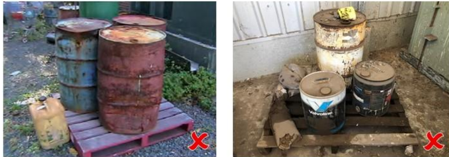
Drums in poor condition, not banded, labelled or covered can leak and contaminate land or water
