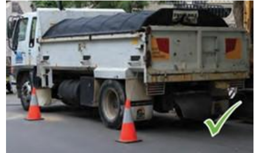
Cover loads to prevent pollution
