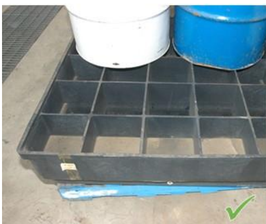
Bunded pallets used for temporary storage of drums
