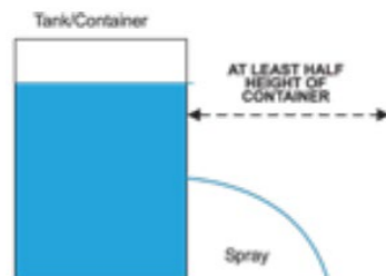
Spray distance is half the height of the container.
